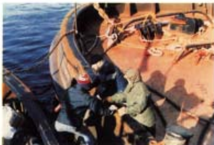
"... and is shackled to a fishplate to which pendants running to each tug's towing cable have already been secured.
