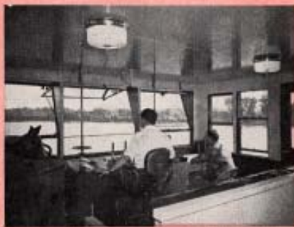
Pilothouse, showing radar scope, search light controls, steering levers, engine controls, Capt. F. Dezendorf and R. Hadley.
