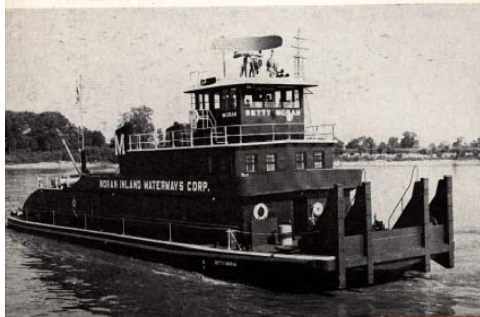
Left: Starboard bow view of our Betty on the Mississippi River below St. Louis. Note characteristic pushing knees and 12-foot radar scanner.
